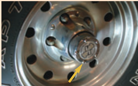
My hubs were of the 5-bolt variety. Be sure to check which yours are, 3 or 5, before purchasing your new hubs. While you are at the parts store pick up a set of "star bit" sockets or wrench (with T-25 Torx) or borrow one from a friend.
