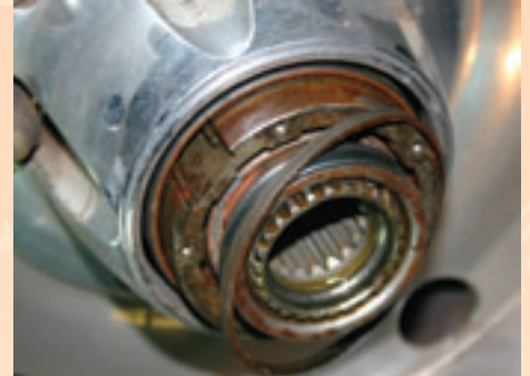
Next use needle-nose pliers to pull out this clip and rubber gasket
