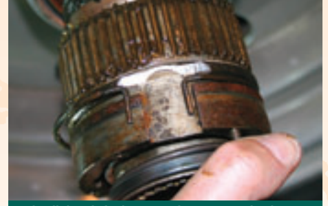
and pull the whole thing out. The retaining clip does not come out by itself, it comes out with the whole thing. A trick is to put a couple of the cover's screws back in the holes to give you something to grab on to.
