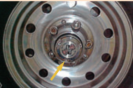
My hubs were of the 5-bolt variety. Be sure to check which yours are, 3 or 5, before purchasing your new hubs. While you are at the parts store pick up a set of "star bit" sockets or wrench (with T-25 Torx) or borrow one from a friend.
