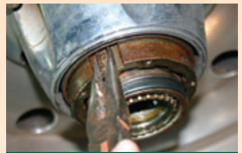
Use the pliers to squeeze the two tabs of the retaining clip together...
