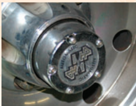
Remove all screws with a T-25 Torx wrench.
