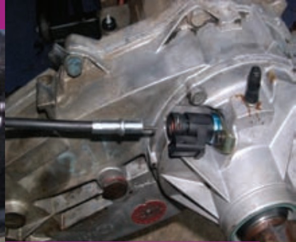
A new speed sensor and speedometer cable from an F-250 replaced the Bronco cable
