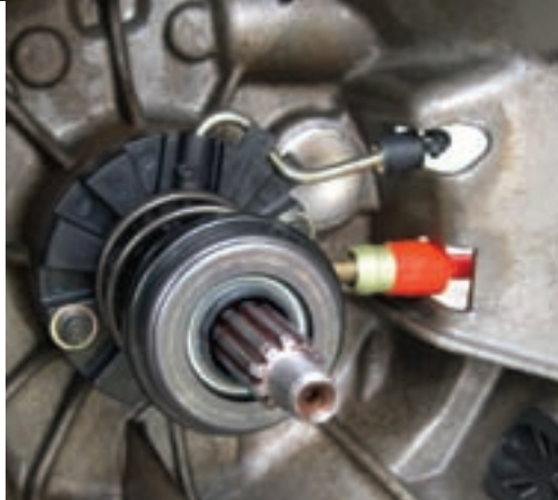
The top line in the picture below is the bleed line and the bottom line with the orange cap quick connects to the line from the clutch master cylinder.
